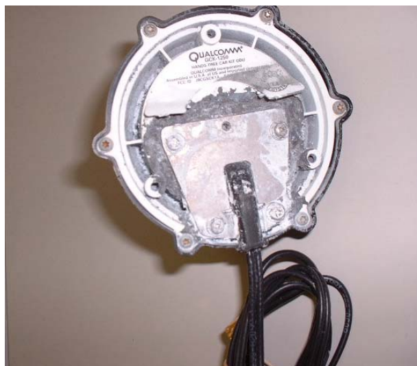
Figure 4. Damage to GCK-1410 antenna from salt water immersion.
